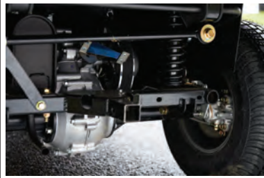
Coil-over shocks suspension for smooth operation
