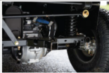
Coil-over shocks suspension for smooth operation
