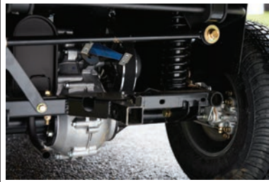
Coil-over shocks suspension for smooth operation
