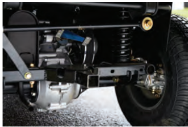
Coil-over shocks suspension for smooth operation
